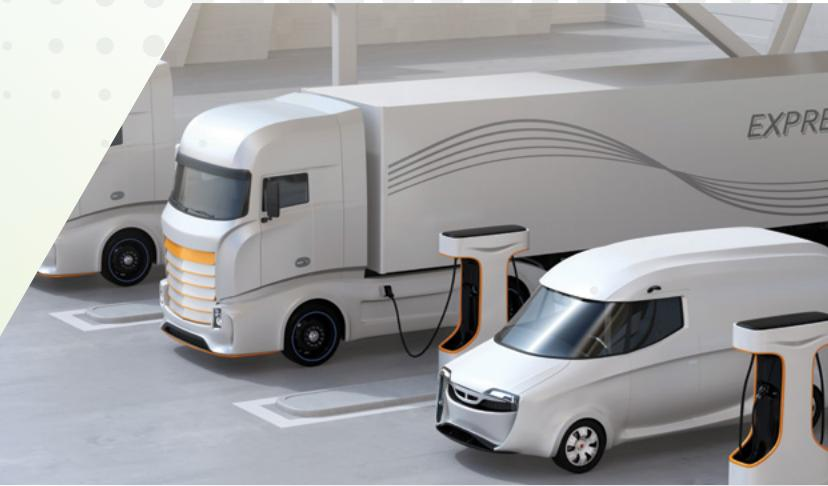
*BEVs are electric vehicles in which the traditional combustion engine and transmission are replaced by batteries and electric motors. The battery size can vary just as fuel tank sizes can vary in combustion vehicles. BEVs rely on electricity as fuel, so they have no tailpipe emissions.*
